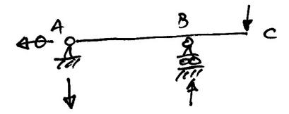
With this information is now becomes easier to establish the bending moment and shear force diagrams. Starting with the bending moment diagram for the portion AB of the beam, we take a cut somewhere to the right of A:
