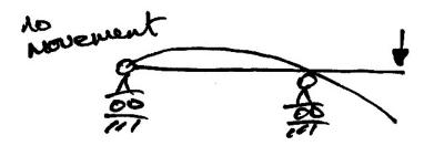
Since there is no movement of the beam when  $H_A$  is released,  $H_A = 0$ .
