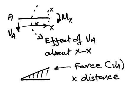
As may be seen, the effect of  $V_A$  is to cause an anti-clockwise rotation of the segment which must therefore be resisted by a clockwise internal bending moment  $M_X$ , as shown. This means (since the arrow comes from the tension face) that tension is on the top of the beam, and is increasing as the distance increases (the force remaining constant).
