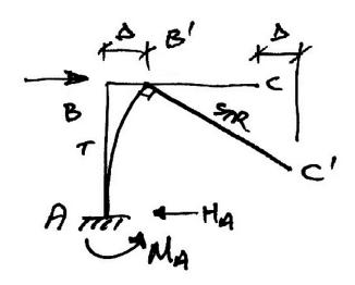
Notice that the diagram emphasises that the horizontal displacements at B and C must be the same since member BC does not change length. Also we see that we develop an anti-clockwise moment reaction at A.
