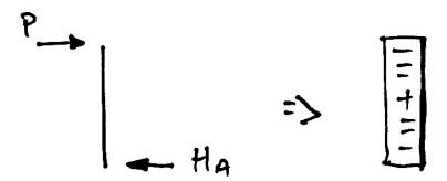
For the shear in member BC, we must first consider that the transverse force (besides  $V_C$ ) gets there through member AB as an axial force (caused by  $V_A$ ), to get:
