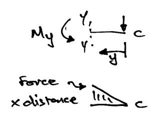
There are no applied moments, so the bending moment diagram does not have any steps in it. This means that the two portions that we have identified above must meet over *B* to give:
