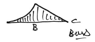
And the shear force diagram follows, either form the load types, or by looking at the BMD (curve to slope, line to constant).
