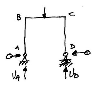
Bending moments are only caused by forces transverse to a member. Thus, with no horizontal reactions (i.e. no forces transverse to members AB or CD), there can be no bending moments in the columns. This only leaves the beam BC to act as a simply supported beam, giving the BMD as:
