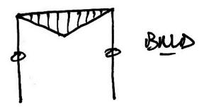
Next we note that the columns are in compression (by the reactions) and transmit the end shears of member BC to ground, whilst there is no axial force in the beam since there are no horizontal forces. The shear force and axial force diagrams are thus:
