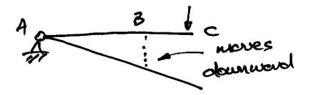
Since when  $V_B$  is removed the beam moves downwards,  $V_B$  acts upwards in the actual structure to ensure that B remains where it should.
