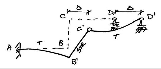
The diagram emphasises the point that the horizontal movement at C and D must be equal since the beam CD does not change length.
