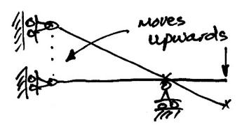
Since when  $V_A$  is removed it moves upwards, it must be that  $V_A$  acts downwards in the actual structure to keep the beam at A where it must remain.
