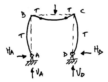
The BMD, SFD, and AFD follow directly by applying the techniques covered earlier given the reactions. Note especially that joints B and C are effectively closing and that beam BC behaves similar to a fixed-fixed beam:
