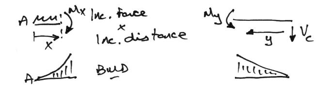
The BMD must not step (no applied moment) and so joins at *B* to yield:
