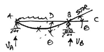
Note that for portion BC we recognize that there is no bending of the member. However, this does no mean that the member does not move: it does, and keeps a straight line extending the tangent to the deflected curve just to the left of B.
