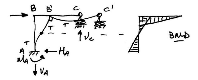
Notice that the *Point of Contraflexure* is noted as a dot in the deflected shape drawing, and its location is produced across to locate the zero point of bending moment on the column AB.
