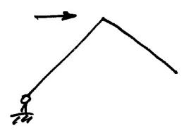
Given this deflected shape, it is obvious that the vertical reaction at C should be upwards to keep C at the correct height. Since there are no vertical loads, this means that because of  $\sum F_Y = 0$ , we must have  $V_A$  acting downwards. Since there is no other possible horizontal force, by  $\sum F_X = 0$  we have  $H_A$  acting to the left. Thus we have:
