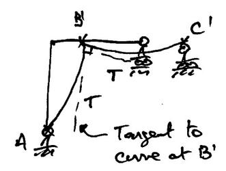
In the above, the tangents to the deflected shape curves are shown at joint B to demonstrate that the joint is rotating, but keeping its angle the same at B.
