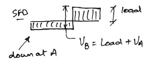
Note also that since V = dM/dx, we see that the negative shear corresponds to a negative slope in the BMD
