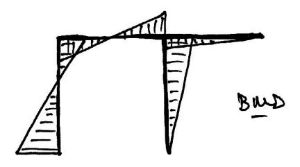
The shear force and axial force diagrams follow similarly by considering the forces along or transverse to each member. One particularly notable point is that the applied horizontal load 'splits' at B: some goes through shear down to A (giving  $H_A$ ), whilst the rest (probably smaller) puts member BC into compression before travelling down member CE in shear to give  $H_E$ . Thus we have:
