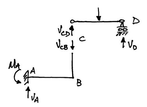
We note then that CD is effectively a simply supported beam, and this gives the interaction force direction as upwards for CD (reflecting the support that the structure ABC offers) and downwards for ABC (reflecting the push coming from the load on the beam). From  $V_{CB}$  we can determine the moment and vertical reactions at A.
